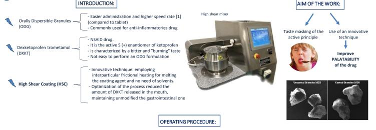
1) Preliminary evaluation: Literature data show the importance of size of the starting product [2]. A preliminary evaluation was made on different particle size fractions of DXKT and Granules with size 180-850  $\mu m$  (M) were selected.
