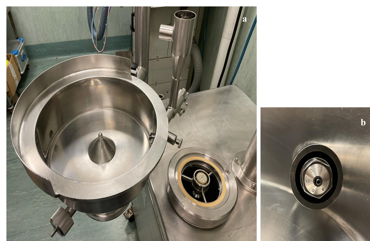
Fig. 4. Photographs of fluid bed equipped with a) rotor insert (tangential-spray) and b) three-way spray system.
