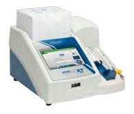
The OsmoTECH XT was designed in collaboration with customers to provide an easy-to-use instrument that can detect osmolality in a wide range of samples. OsmoTECH XT uses Intelligent freezing technology to monitor, control and measure samples with high concentration/viscosity. The instrument is ideally suited for laboratories that need to measure a wide variety of sample types across bioprocessing and cell and gene therapy workflows.
