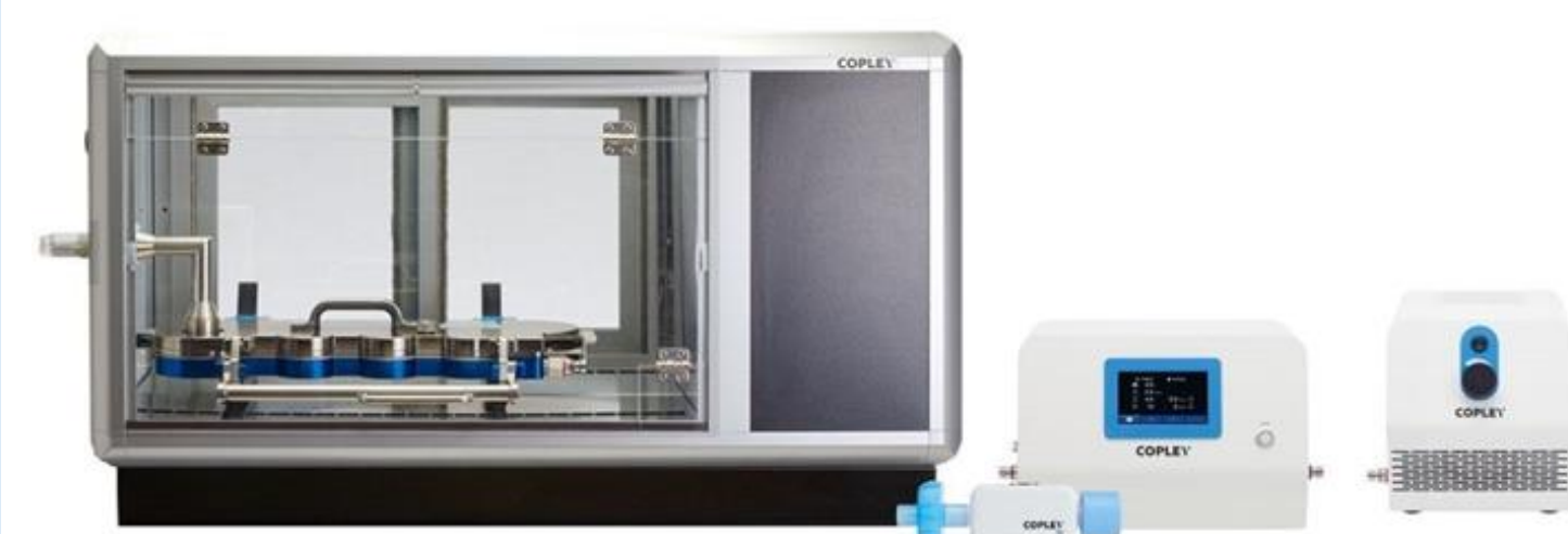
NGI inside the cooler and connected to the breath actuation controller and the low capacity vacuum pump, respectively
