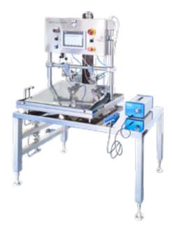
BRAM-COR manufactures bags linear filling equipment Mod. **BFIL** according to CGMP regulations. The equipment is completely validable with all parts in contact with the fluids in AISI 316L mirror polished S/S and with PLC controlled electronics. Upon request it is possible to modify the software and thus the operation of the machine including vacuum extraction, gas or sterile air injection, etc.
