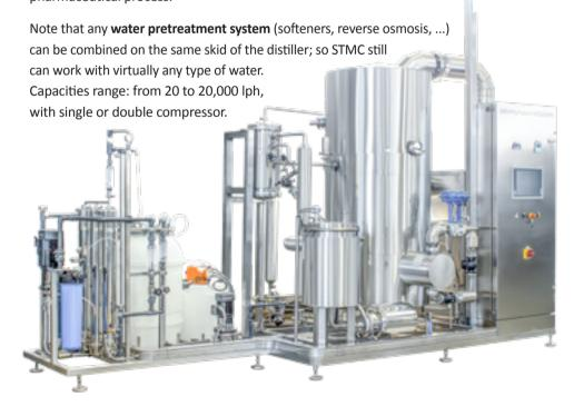
STMC vapor compression distillers can operate with electrical heating or with steam heating or a combination of the two (electrical and steam heating systems). STMC distillers can produce both cold distillate at a defined temperature and hot distillate with huge savings of energy costs and without the need of cooling water. The design,
