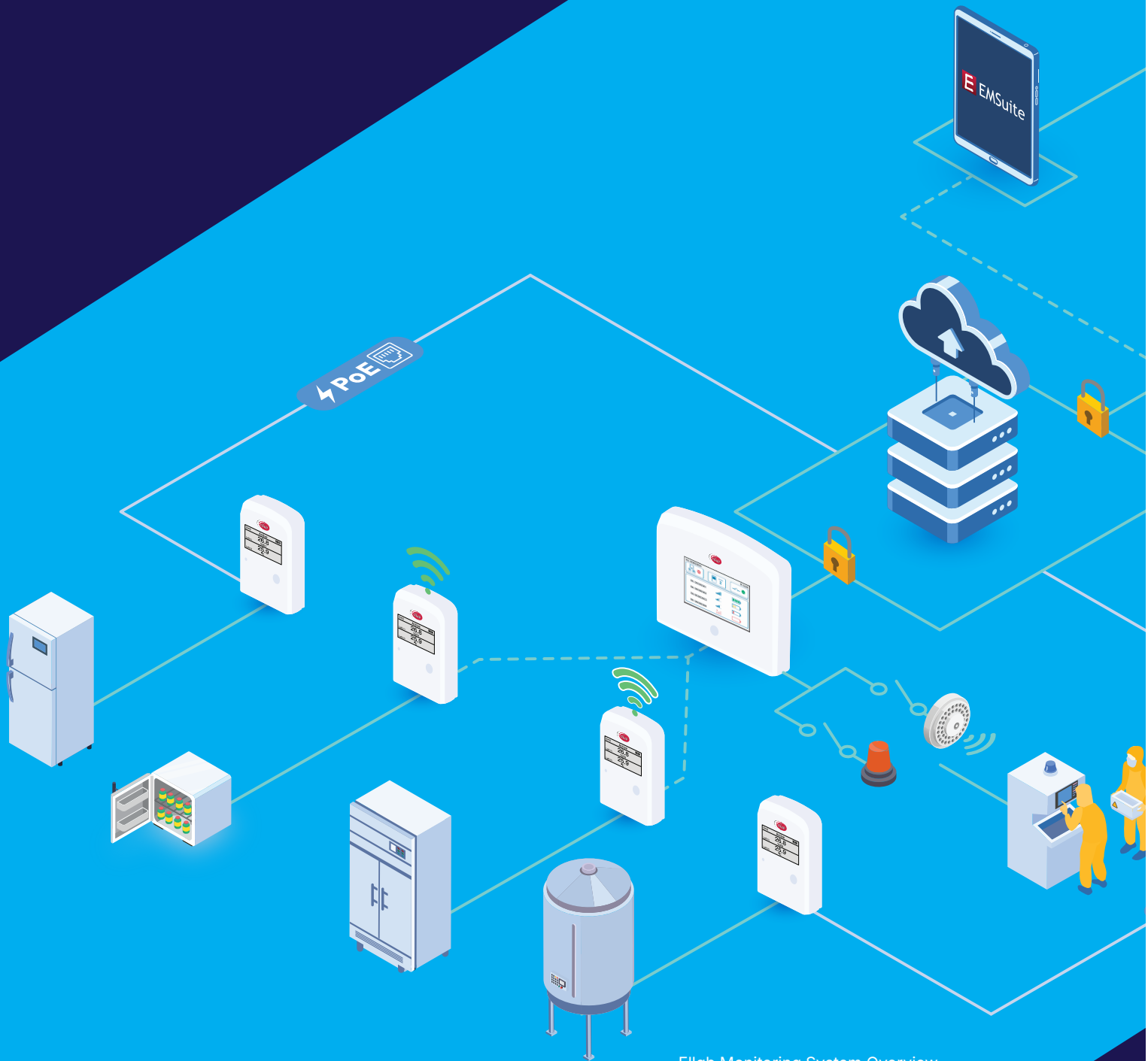
Ellab Monitoring System Overview
