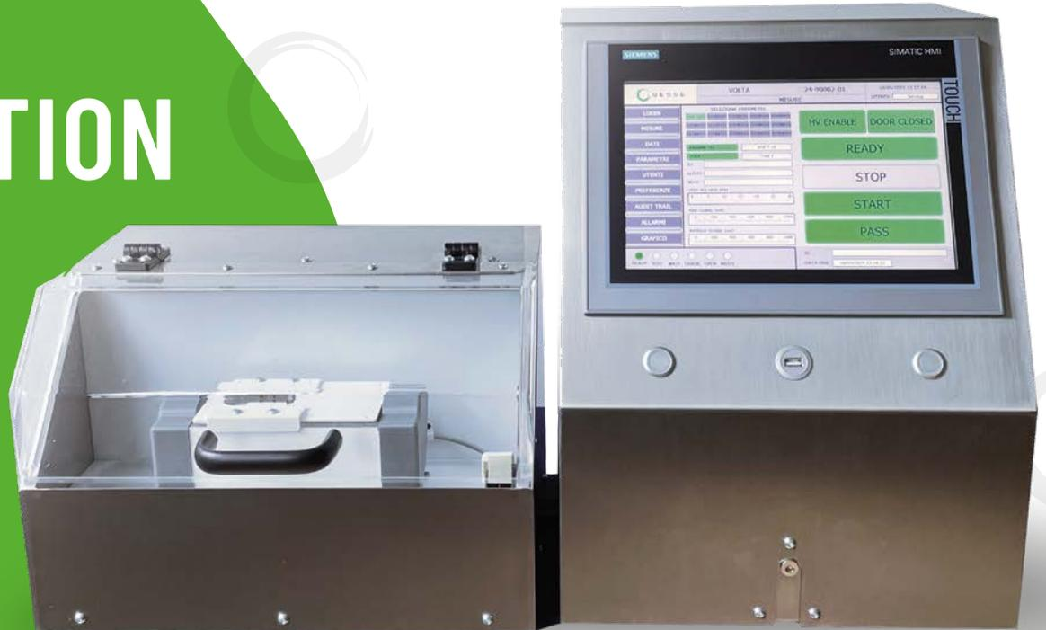
QESSE **VOLTA** is a nondestructive High Voltage Leak Detection (HVLD) bench top unit for package integrity testing on your liquid filled containers.
